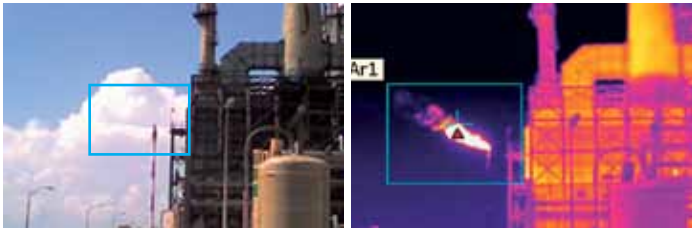
A thermal imaging camera can monitor flames that are invisible to the naked eye. Note that the flare is invisible on the visual image.
