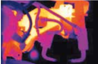
Hot spot in welding robot
