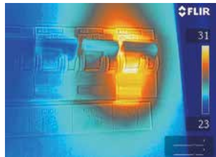
Thermal image of the same overheated fuse, now using the MSX-setting. The text below the fuse is readable, making it very easy to identify and repair the correct fuse.
