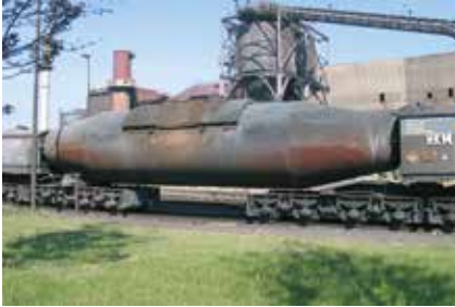
A visual and thermal image of a torpedo ladle.
