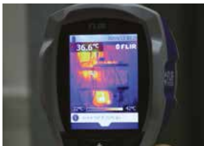
A thermal imaging camera can be used to inspect many different devices.
