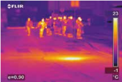
A leak in the underground hot water pipeline can be clearly located thanks to thermal imaging.
