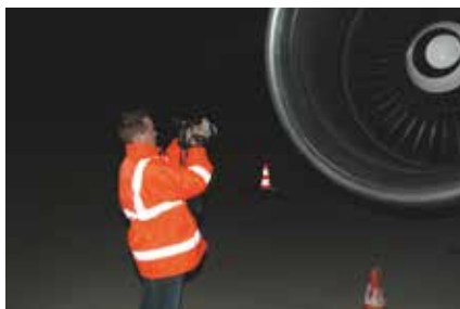
Inspecting an airplane with a FLIR thermal imaging camera.
