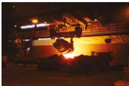
The refractory on this ladle shows signs of wear and if it degenerates further needs to be replaced. Thermal imaging cameras are the only practical tool available for refractory inspections.
