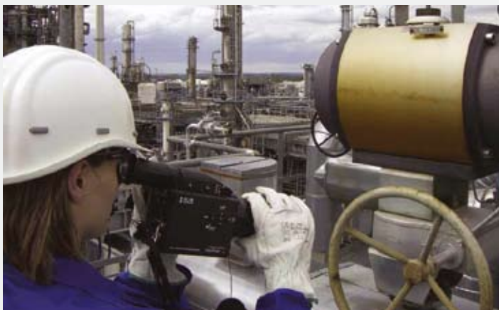
Examining potential leak paths
