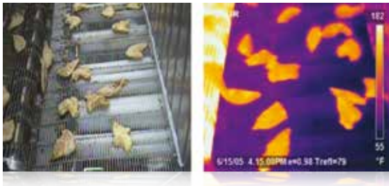
Figure 6. An IR temperature measurement and thermographic image are used to locate undercooked chicken tenders and stop the line so bad parts can be removed.
