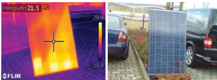
A test with a solar panel shows that the hot spots can quite easily be seen on the thermal image, even from the front.
