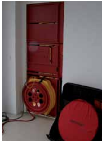
The 'BlowerDoor' equipment is normally installed in the entrance door.
