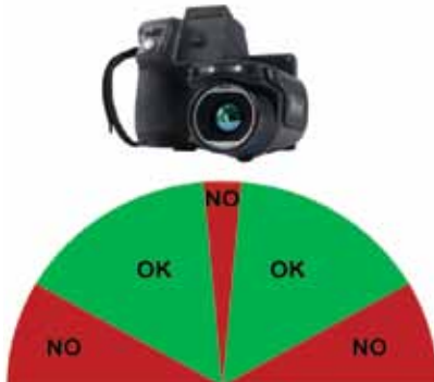
Viewing angle recommended (green) and to be avoided (red) during thermographic inspections.
