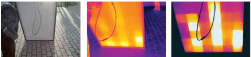
Images taken from the back of a solar panel show much less reflection than the front, making the temperature measurements much more accurate.
