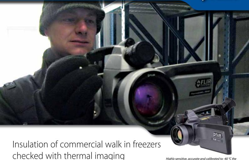
Highly sensitive, accurate and calibrated to -40 °C the FLIR P640 thermal imaging is the perfect tool for freezer insulation inspections.
