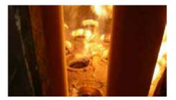
Inspection ports provide a view of internal parts, but flames, combustion gases, and ash obscure the equipment during operation. A FLIR thermal imaging cameras with a flame filter is not hindered by such obscurants.
