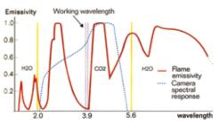
The small grey area indicates the part of the spectrum where the combination of high camera sensitivity and low flame emissivity makes it possible to see through flames. Because everything but that specific part of the spectrum is filtered out, the thermal imaging camera can now see through the flame and make temperature measurements straight through even exceptionally hot flames. This makes thermal imaging cameras equipped with such a filter ideal for furnace inspections.
