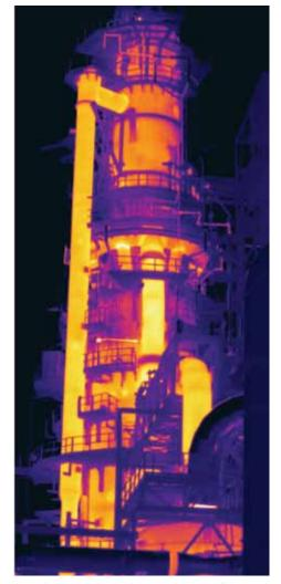
According to Tournieux the FLIR P640 can still detect small hot spots from a large distance indicating insulation failure.
