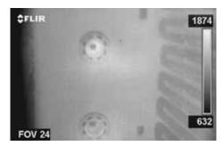
Due to the built in flame filter the FLIR GF309 thermal imaging camera can see through flames and even measures the temperatures behind the flames.
