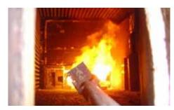
The thermocouple probe is inserted in the furnace. Tournieux then uses the temperature reading to accurately correct the thermal imaging camera for emissivity.
