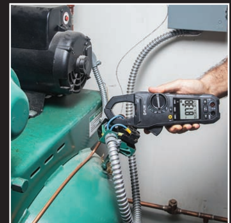
Inrush Current detects start-up current spikes
